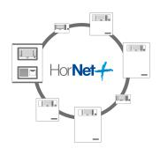
In order to enlarge the installation, it is possible to connect several Previdia Max and Previdia Micro control panels (with a maximum of 48 points including control panels and repeaters) thus creating an expanded system (Hornet+network).
