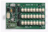
The EM500 module allows you to create a synoptic panel by means of an overlay which attaches to the panel front. This is done by perforating the overlay in the positions which represent the zones and wiring up the corresponding LEDs by means of the wires supplied with the board.
